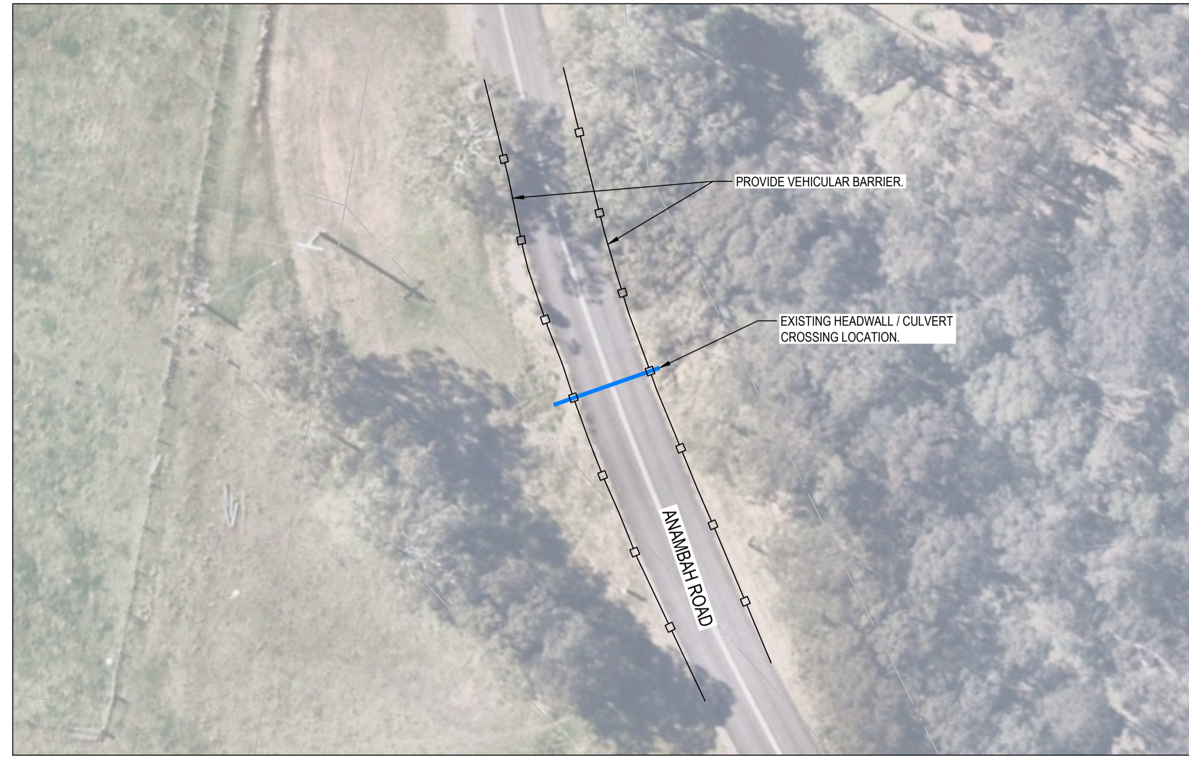
ITEM 14 - UNPROTECTED EMBANKMENT (CH0-100)
